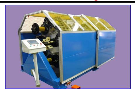
AWM Rigid Stranders are designed to produce cables of up to 24 single wires or single fibers in a single pass. Tandem configuration of two 12-reels sections allows for cables of multiple configurations up to 24 single wires or fibers in two layers in a single pass.
