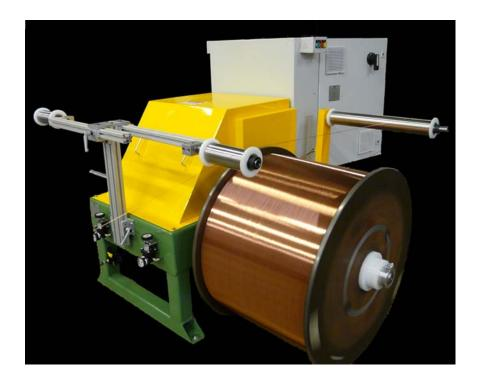
AW Machinery Shaft Buncher Payoffs, Model SBPO-2-XXX-M are motorized Machines with integral Dancers and they are designed to process two reels in a single machine.
